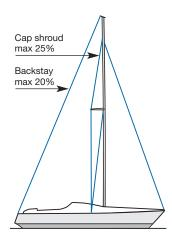
In general, this type of rig needs more tension in the shrouds than a rig with in-line spreaders. The tension in the forestay is affected by three components;
