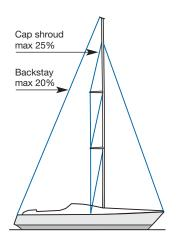
This type of rig is very demanding on the sailor, since it is complex to tune and to handle. In general, this type of rig needs more tension in the shrouds than a rig with in-line spreaders. The tension in the forestay is affected by three components;
