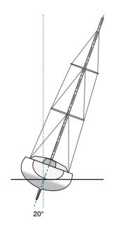
Fractional, in-line multi-spreader rig, deck-stepped mast, forward and aft lower shrouds. Alternatively baby stay and aft lower shrouds.
