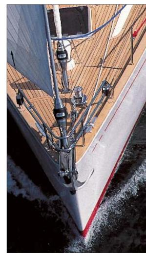
Furlex comes in five sizes, 100S, 200S, 300S, 400S and 500S, and is suitable for yachts ranging from 25 to 70 feet.
