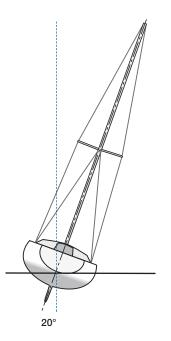
Masthead, multi-spreader rig, swept spreaders, deck-stepped mast, forward and aft lower shrouds. Alternatively baby stay and aft lower shrouds.
