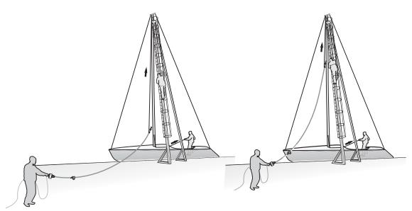
Normally, the jib furling system is placed on the forward side of the mast when the mast is being lifted by the crane. One person is detailed to prevent the system damaging the mast or yacht. The extrusion used in the furling system can cope with large radius bends without any problems, but may break in the event of uncontrolled buckling.
