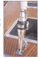
motor is located inside the worm gear, as on the in-mast furling system. The positioning of the motor contributes to the compact design of the Furlex Hydraulic.
