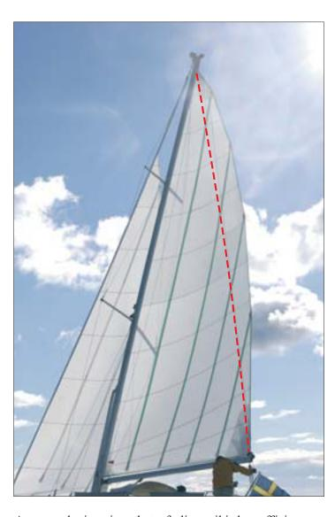
Anyone who imagines that a furling sail is less efficient because it cannot provide sufficient roach would be wrong. The new Seldén in-mast furling masts are made for vertical battens and a true positive roach.
