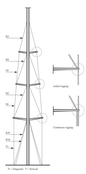
**Cap shrouds:** (V1-V3, D4) Stay the mast against lateral (athwartship) loads. Attached near the masthead on a masthead rig, and at forestay level on a fractional rig. The cap shrouds are led via spreaders to the boat's chain plates.
