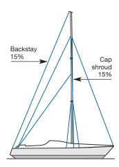
Runners are required to give sufficient longitudinal stability, and to obtain the required forestay tension. The backstays must be located as near the centre line of the hull as possible so as not to affect the lateral tuning. This type of rig is also found with single lower shrouds, in-line, and in that case checkstays are recommended to prevent excessive mast bend.
