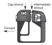
Clamping end plug for continuous rigging.
