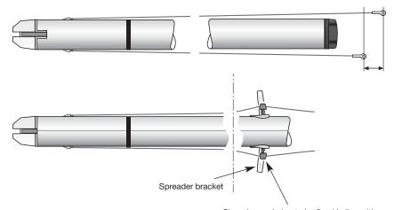
Clamping end plug to be fixed in line with spreader brackets, with shrouds tensioned along the mast. Final vertical spreader angle must always be 6°.
