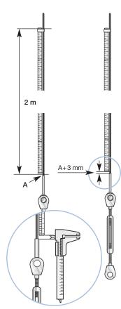
Hint! Count how many turns on the rigging screw corresponds to 1 mm elongation (5% of the breaking load). Make a note of it. This is useful to know if you ever need to tension "another 5%".
