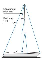
This type of rig is very demanding on the sailor, since it is complex to tune and to handle. In general, this type of rig needs more tension in the shrouds than a rig with in-line spreaders.
