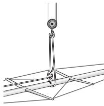
Lifting strop secured at the mast's centre of gravity.
