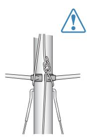
Make sure the strop does not interfere with the lower shroud attachments.
