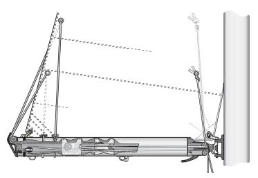
It is important to note that no fittings should be mounted on the sides of the booms. The space between the carriages for the running blocks and the sides of the boom is limited. Fastenings for external fittings could prevent the movement of the carriages.
