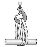
Lift hook with locking device and endless lifting strop.
