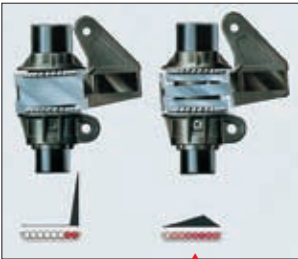
Seldén patented load distributor.
